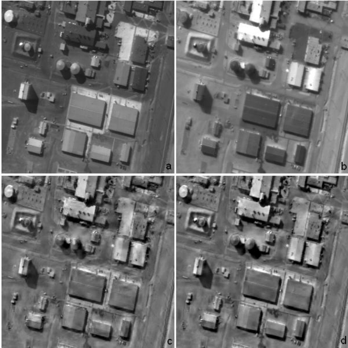
Figure 5: Input images a) and b), signal-level c) and multi-level d) DWT image fusion
